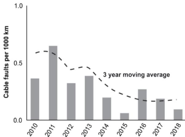
Fig. 9. Cable faults in <1000 m water depth have generally declined into the present mainly in response to improved armouring and cable burial. Based on data from Kordahi et al. (2019).
