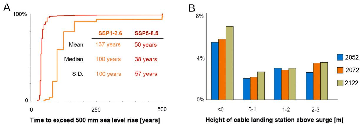
**Fig. 4.** Projected sea-level at cable landing stations. (A) Proportion of cable landing stations where sea-level rise is projected to reach >500 mm above present day levels within different timeframes under two IPCC sea-level scenarios. (B) Elevation of cable landing stations (expressed as a percentage of cable landing stations globally) above a 1 in 100 storm surge for the IPCC SSP5-8.5 scenario.
