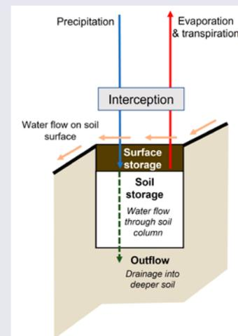
Figure D1 Illustration of conceptual hydrological model. Figure © BGS-UKRI.
