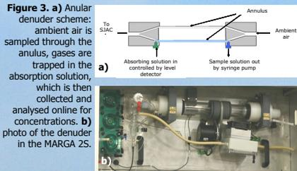
**Figure 3. a)** Anular denuder scheme: ambient air is sampled through the annulus, gases are trapped in the absorption solution, which is then collected and analysed online for concentrations. **b)** photo of the denuder in the MARGA 2S.
